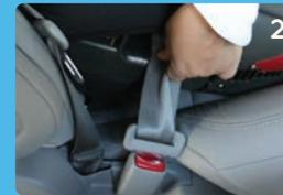
Place the seat in the car, feed the seatbelt through the tunnel and guides and secure the buckle.
