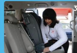
Push the seat down, tighten the belt and secure with the lock off clip.
